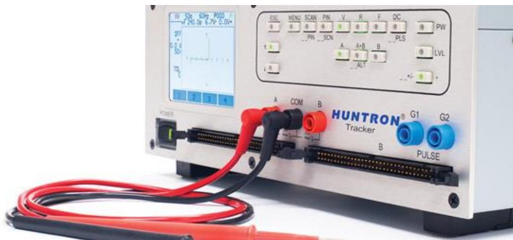
**Picture 3: Huntron Tracker 3200S** as a stand-alone desktop unit. Easy to use with a user-friendly touch screen, and a 128-way scanner.
