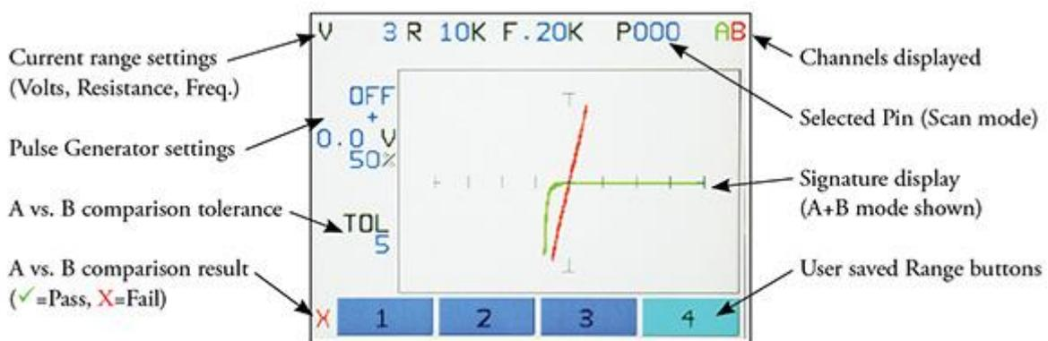
Picture 2: ASA Signature Display: The picture of the defective test (red), in comparison to the "golden" reference (green).
