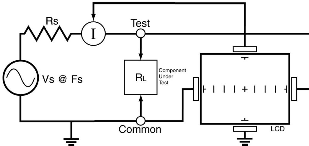
Picture 1: Block diagram of the ASA
