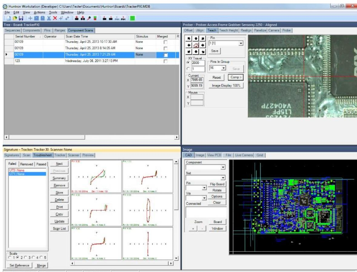
**Picture 5: Huntron Workstation Software** clearly presents the test instructions on the board, the test sequence, and component/pin level test results. It also allows user guidance with integrated illustrated work instructions.
