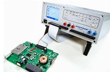
Additional synchronous pulse generators can be connected to the controlling input of a component. This allows the testing of active power components, such as relays, triacs or transistors.
